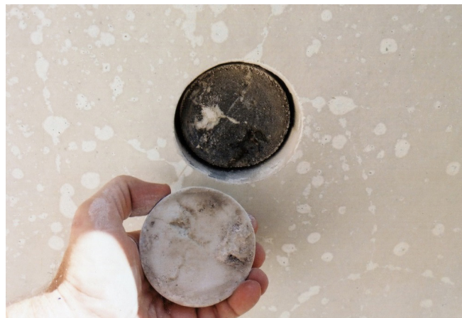
Figure oB-00015a – Bond Failure and Cavity Behind Crack and Nodule
