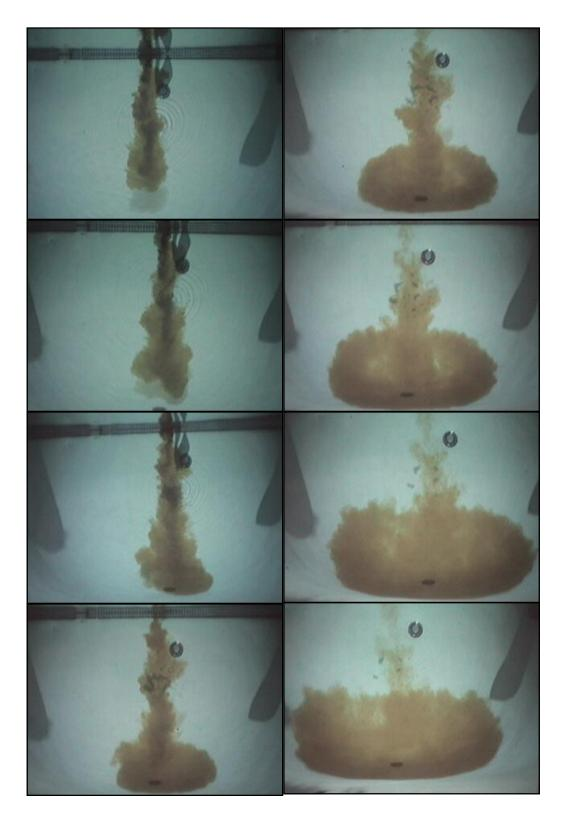
This sequence of photographs was taken in Livermore, California and shows the path of the muriatic acid (colored with phenol red dye) from the point of application to the puddle. For these photographs, a single quart of acid was used. The puddle remained well defined for more than 25 minutes, and was dispersed at that time by turning on the circulation system. The pH in the puddle was 2.1, and the pH inches away from the edges of the puddle was unaffected.
