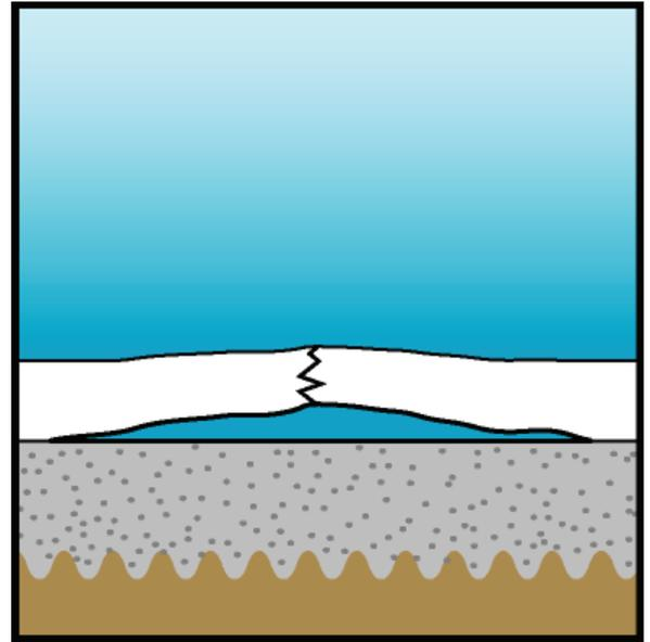
5. Interior pressure generated by the “calcium/pH factory” pushes a “plume” of high pH, calcium hydroxide-rich water out the “smokestack” or crack/perforation in the plaster.
