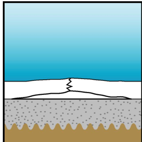
4. Gradually, water from the pool penetrates the void via the hole or crack, and creates a localized chemistry environment completely separate from the water balance in the pool. As calcium hydroxide bleeds into the void water it creates a calcium-rich, high pH solution like a little “calcium/pH factory” beneath the plaster surface. The pinhole or crack is not of sufficient size to create a rinsing effect like that going on at the plaster surface.
