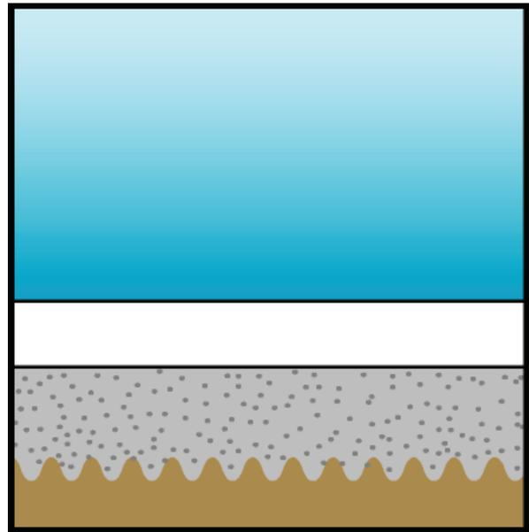
2. Sometimes, an air cavity can be formed between the gunite and the plaster. This is referred to as “delamination” and the cavity is referred to as a “void.” As long as the void is not connected to the surface of the plaster, the fact that the void even exists may not be known. Unless the plaster completely separates from the surrounding plaster, creating what is referred to as a “pop-off,” this is not considered by the plaster industry as a defect.
