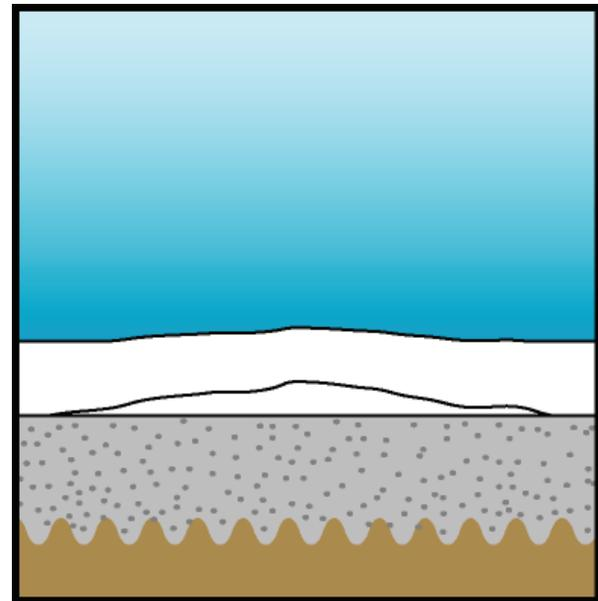
3. In some cases, however, the void is connected to the surface by a small pinhole or hairline crack.
