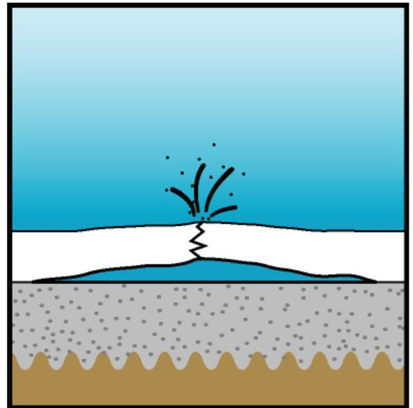
6. As the plume solution comes in contact with the pool water at the plaster surface (which, if balanced, is bicarbonate-rich because of the alkalinity and balanced pH) the material is converted to the carbonate form, and builds up a “slag pile” of calcium carbonate around the exit point. This point has been referred to as a “point of attachment” but could more properly be referred to as a “point of hydroxide egress” or “calcium supply point.”
