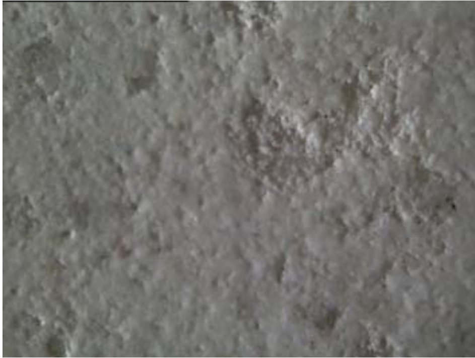
Figure 18 – Aggregate Exposure of Plaster Cured in Balanced (Non-aggressive Water)
