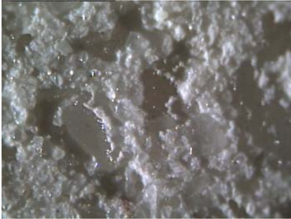
Figure 20 – Aggregate Exposure of Moderately Etched Plaster
