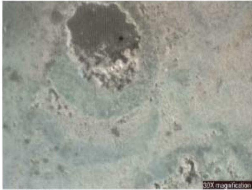
Fig. 1 Stereomicroscope image showing soft spots over marble aggregates and discoloration of the troweled surface of the plaster.
