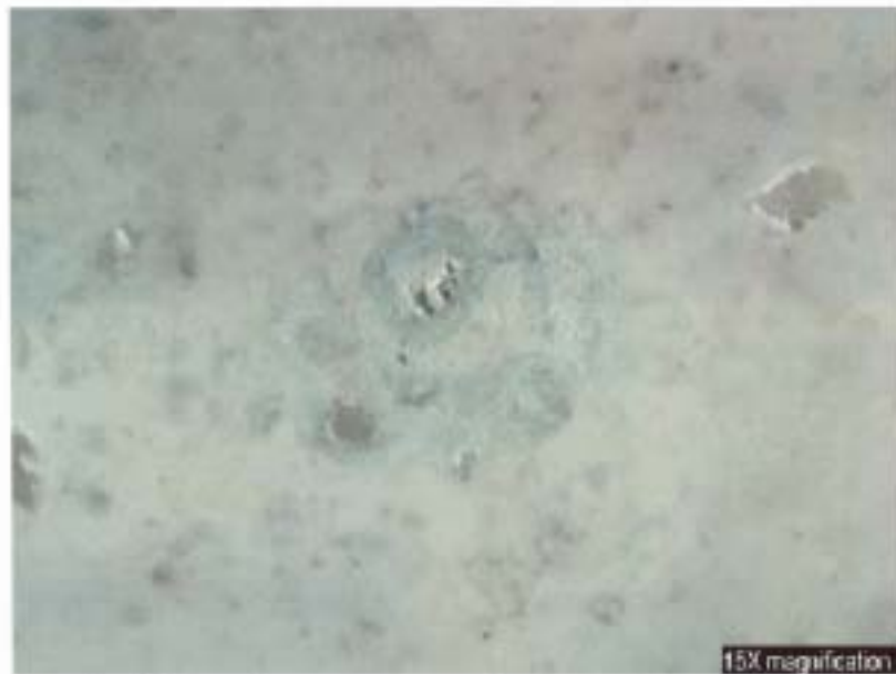
Fig. 2 Stereomicroscope photograph showing soft spots and discoloration on the troweled surface of the plaster.
