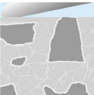
Since the plaster is drying so fast, the plastering crew needs to “knock it down” smooth, sometimes with late, excessive hard troweling.
