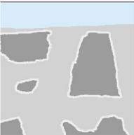
The sand doesn't shrink – just the cement paste around it shrinks and pulls away from the sand.
