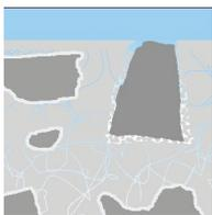
Leaching then spreads laterally through the micro-cracking fissures, forming the characteristic round spot. This can continue until many spots coalesce into bigger spots.
