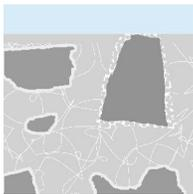
As the water dries, it leaves behind a loose latticework of crystalline calcium hydroxide in its place.
