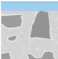
...water penetrates the area around the sand grain and leaches the weak material away. This leaching is due to the solvency of even perfectly balanced water – although it happens faster because of the inferior, compromised paste.
