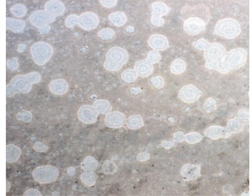
**How does it happen?** Over-accelerated (and thus porous) plaster is late hard troweled, disturbing aggregate at surface. Water-troweling allows water to penetrate the paste-to-aggregate interface. Over time, water in the filled pool leaches soft paste from around the surface aggregate, and continues leaching in a pattern radiating from the point of origin.
