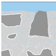
Aggressive water will make the process happen faster and maybe deeper, but the defect ensures that the spot will form even in perfectly balanced water.
