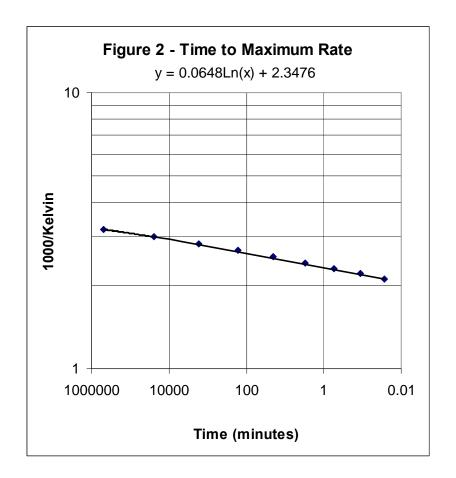
straight line with slope  $R/\Delta E$  (see Figure 2). Linear regression can be employed to obtain an equation of the line and allow extrapolation to lower temperatures. The temperature at which the value of  $t_{mr}$  equals the time constant t is equal to the critical temperature  $(T_a)$ .
